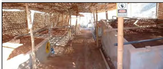
Artisanal miners can do safe and efficient cyanide leaching. Processing plants like the one in Santa Filomena (Peru) require considerable investment and care, but leads to mercury elimination.
